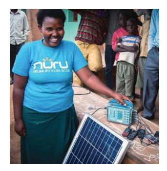
(VLEs) to sell rechargeable Nuru Lights and fee-forservice recharging via a 60 watt solar panel or the company's patented POWERCycle pedal-powered generator. Both the solar panel and POWERCycle charge Nuru's Octopus Charger portable recharge box, which can subsequently charge up to five mobile phones or five Nuru Lights simultaneously in 20 minutes – with each light lasting 28 hours.
